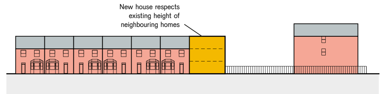
Fig. 120: New street extension should generally respect the height of the street they are extending.
