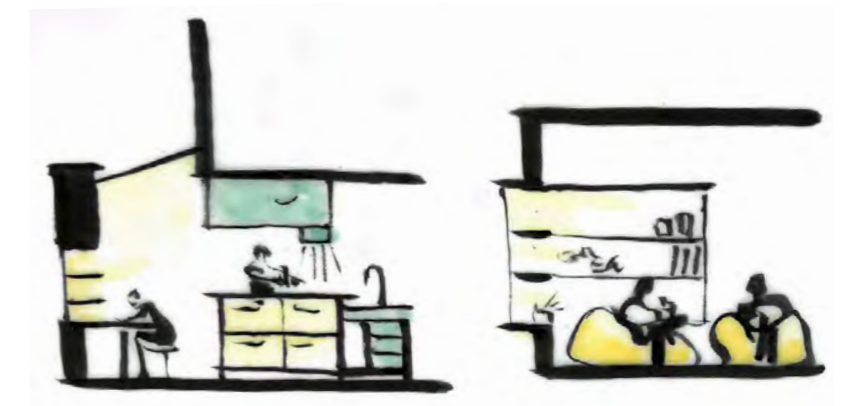
Fig. 49: High ceiling and large fanlight, good daylight to worktop and desks, well-lit living areas
