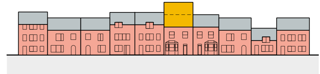
Fig. 153: In most cases, where neighbouring buildings are of varying heights, a modest increase in individual properties will be supported where these result in a net increase in the number of dwellings.
