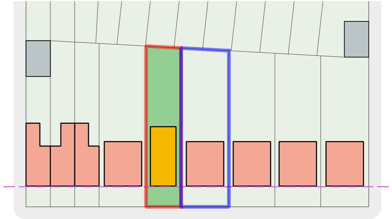
Fig. 98: A large plot occupied by a single detached dwelling can be sub-divided into two smaller plots to make way for a new infill development.
