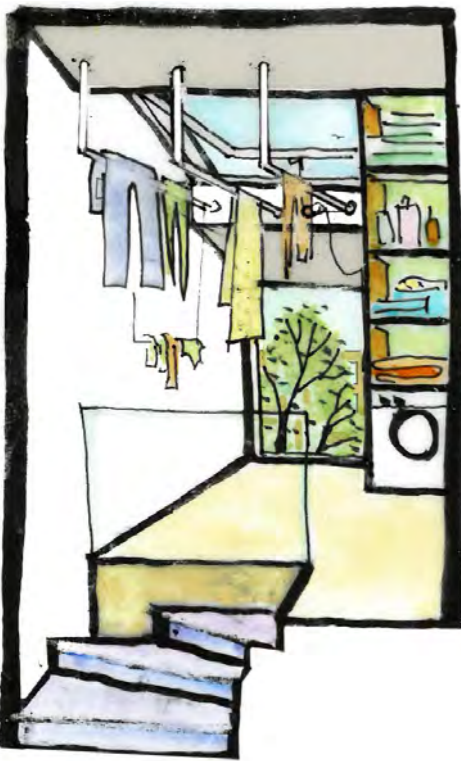
Fig. 46: Skylight over a laundry landing
