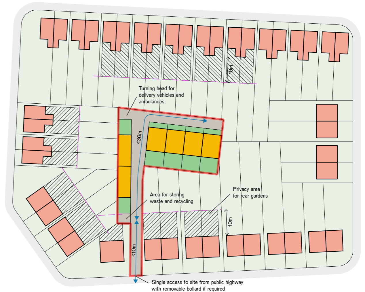
Fig. 173: The development of backland garage sites can provide high-quality new homes, provided that these are carefully designed and respond positively to their context. In most cases, access and parking space for private cars will be resisted.
